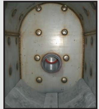
Weekly cleaning allows for optimal performance. The easy access front and rear inspection doors along with included ash scoop and rake make cleaning fast and convenient.
