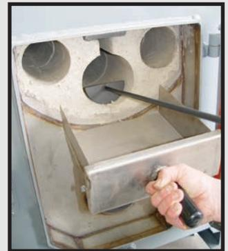
A high velocity draft fan moves air through the wood allowing for easy cold start up. After the gasification process begins this air movement produces intense flames and very high temperatures in the gasification tunnel. In turn The air flows through the heat exchanger cleaning as it passes through.
